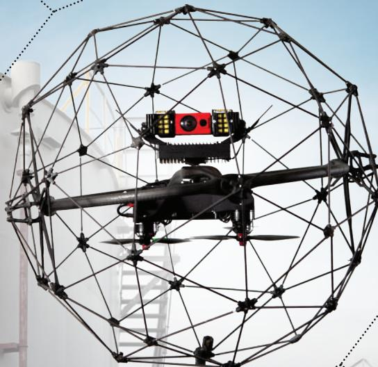
THE COLLISION-TOLERANT UAV
